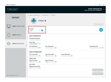
$<sup>^2</sup>$  You can check device's serial port name in "Device Manager" on Microsoft  $^\circ$  Windows  $^\circ$  operating system.
