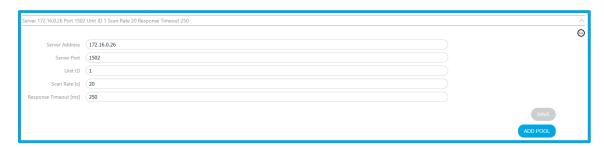
Figure 138 - Modbus TCP/IP window section to configure the server.
