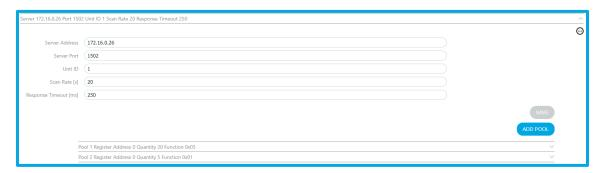
Figure 140 - Modbus TCP/IP window section to configure server requests.
