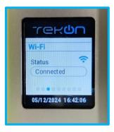
Figure 117 - uGateway display showing the Wi-Fi connection status.
