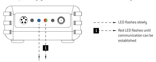
• The Repeater is connected to the wireless network when red and green LEDs flash.
