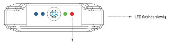
• The *Transmitter* is connected via wireless and its data is available in the *Gateway*, when the red and green LEDs flash.
