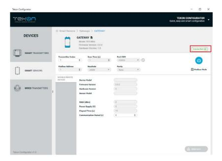
The messages *Connected to Modbus* and *Reading successfully* will appear if the *Serial Port* configuration parameters are correct and the Modbus connection established.
